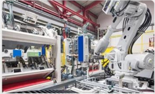
Robot spray mould release agent and injection PU raw material
