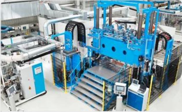
KRAUSS MAFFEI High Pressure Reaction Injection Molding (RIM) Machine from Germany
