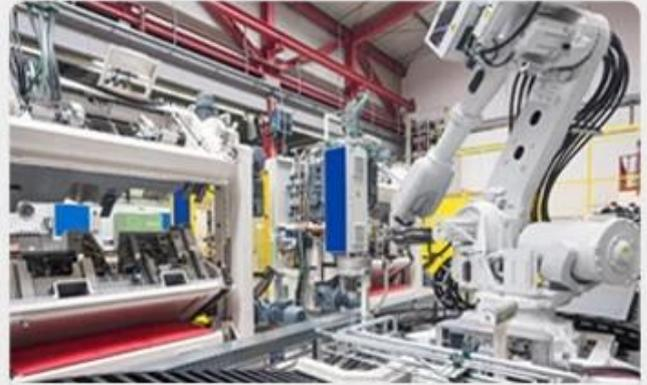
Robot spray mould release agent and
